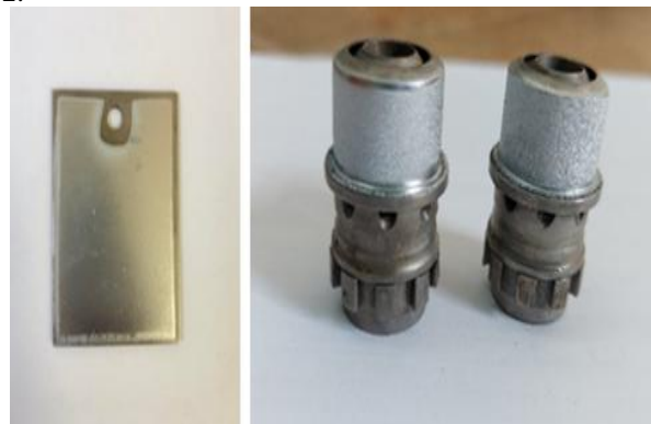
Figure 2: The appearance of the standard plate and shroud-fuel nozzle after the hard chrome plating process
